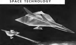
ARTIST'S conceptions of how a pointed aircraft might use reflecting planes to reflect wave drag. Flow fields originating on the forward wing surfaces would be reflected against the rear surface and produce thrust. Possible planes reflecting waves would approximately define only Mach 10 region to keep the proper spacing between the surface and the aircraft.
